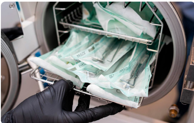
Above: Don't overload autoclaves! Lay packets in one layer on each tray.
