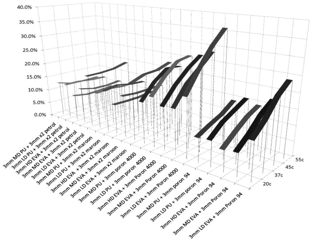
Figure 1. Rebound ratio at different temperatures for different material combinations.
