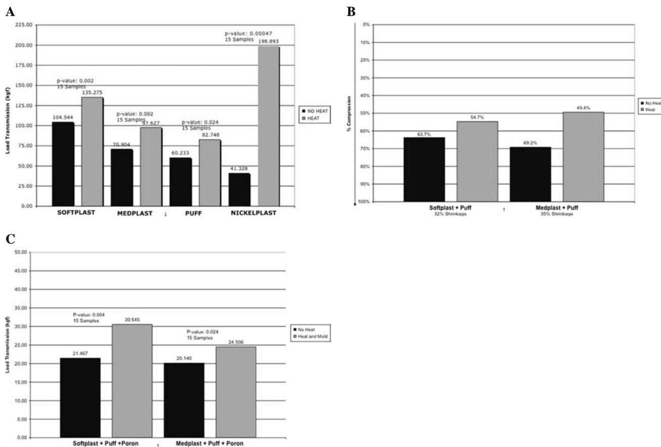
Fig. 4: Load transmission: (A) individual materials; (B) two-material combinations; (C) three-material combinations.
