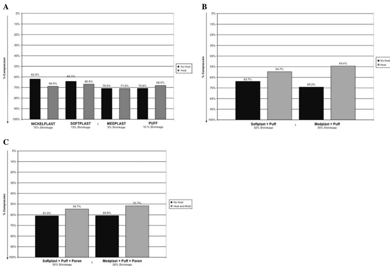
**Fig. 2:** Percent compression: (A) individual materials, nonheated versus heated; (B) two-material combinations, nonheated versus heated; (C) three-material combinations, nonheated versus heated.
