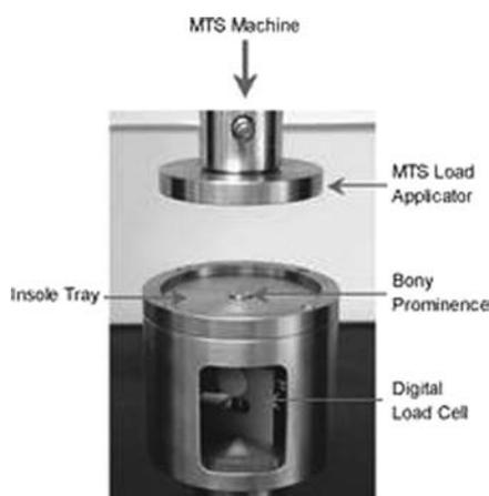
**Fig. 1:** A MTS load applicator and a digital load cell were attached to a custom-made stainless steel testing jig to test the insole materials.
