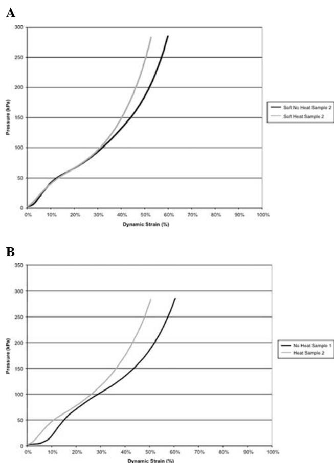
**Fig. 3:** Stress–curve: (A) soft Plastazote + Puff + Poron; (B) medium Plastazote + Puff + Poron.
