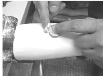
7) Apply a slurry of plaster around the sides of the TL-100 to fill in all voids beneath the light module.
