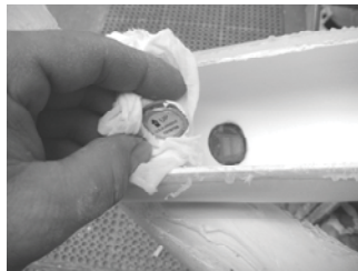
13) Once plastic is cooled remove orthoses from mold and strip away the nylon. Depending on the amount of vacuum pressure used- the light will sometimes easily dislodge from plastic.
