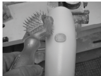
11) Re-apply the foam interface to the positive cast and then use a perforating tool to optimize vacuum.
