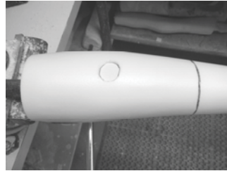
3) Carefully remove the cut out from the mold.
