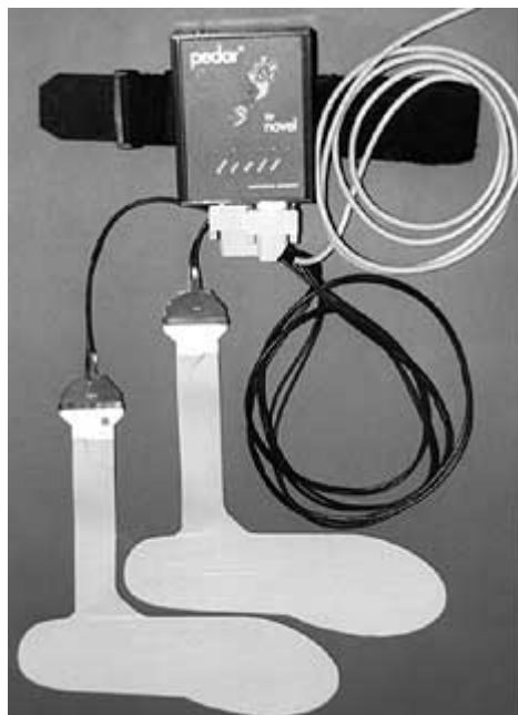
Figure 1. The EMED Pedar System (Novel USA, Minneapolis, MN) used for in-shoe pressure measurements.
