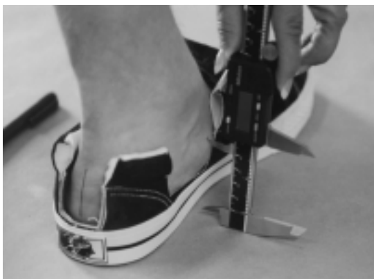
Figure 5: The use of the digital callipers to measure changes in the height of the navicular with the use of the different foot orthoses.
