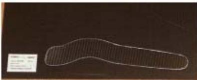
3. - Heat the material with a heat gun @ 630 C with a sweeping motion.
